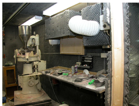
Sound insulation, air ventilation and a purification system are present inside this mobile tableting unit. Photo: Europol.
