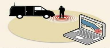
By collecting signal strength in several locations, the system can triangulate and map a phone's location.
