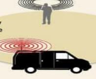
Often the device is used in a vehicle along with a computer with mapping software.  The stingray system, which mimics a cellphone tower, gets the target phone to connect to it.
