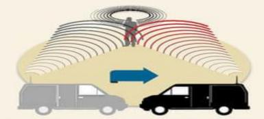
The vehicle can then move to another location and again measure the phone's signal strength.
